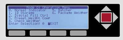
of Operation. You can then access other ID-related set-up screen like ID Counter by answering follow-up questions. The 225 Navigator does the rest by configuring the normal operating screens such that each operational step associated with ID Storage is located within the four soft keys.
